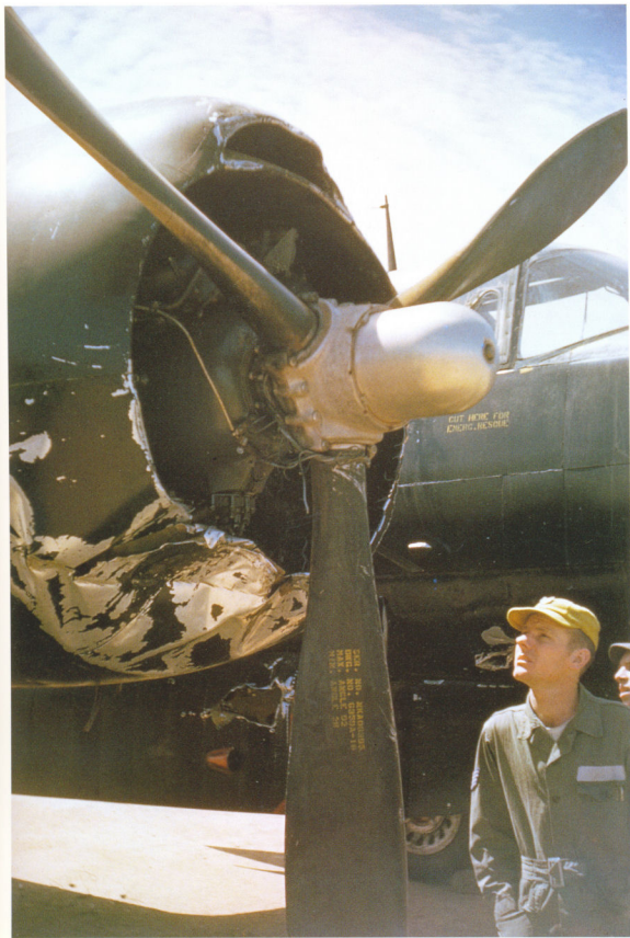
LEFT In an effort to deter UN aircraft from strafing, the North Koreans stretched thick steel cables between a number of the narrow valleys 'up north'. Despite communist hopes that unsuspecting fighter-bombers would hit the cable and crash, this particular B-26 flew through a wire and just kept right on going! However, on other occasions F-51 Mustangs and at least one F-82 were brought down by the cables, with the respective pilots being killed (HA Gamblin)
